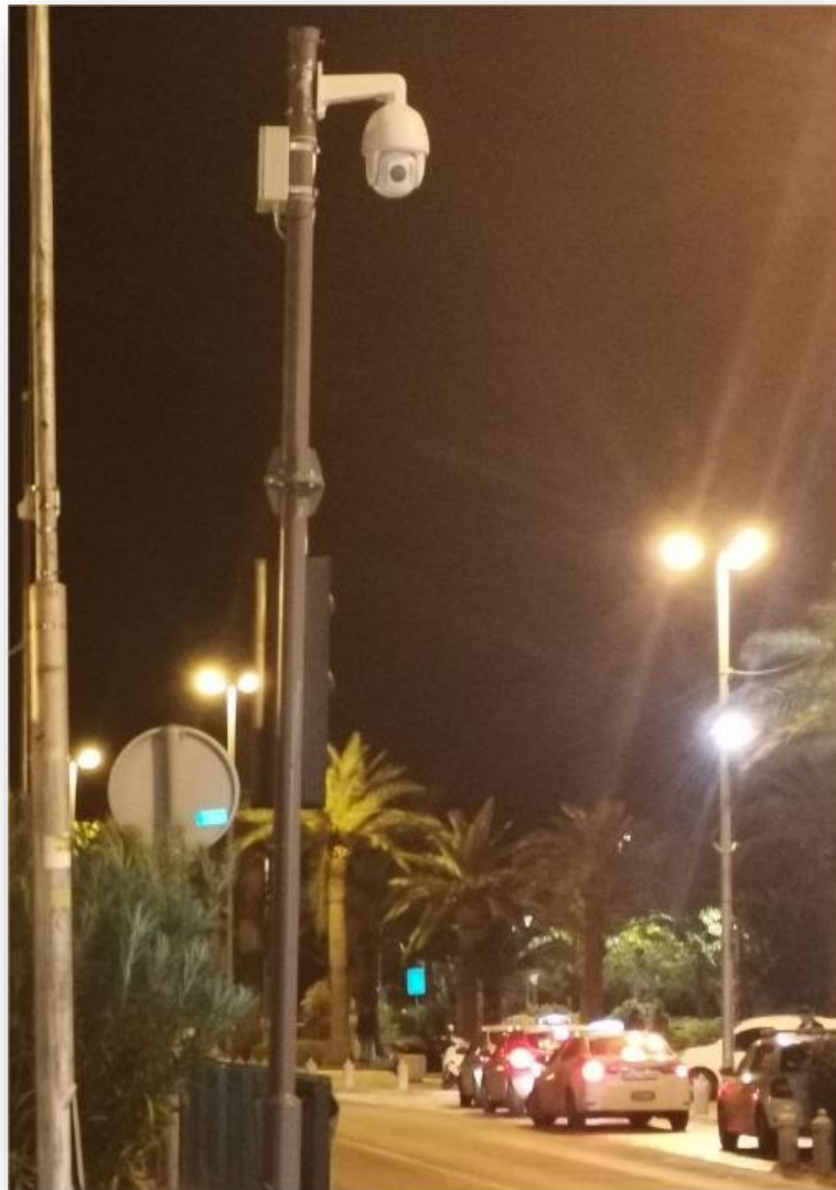
Figure 57 : Good Practice A – A smart system to identify car plates, evaluating visitors' origin and flows (A9)
